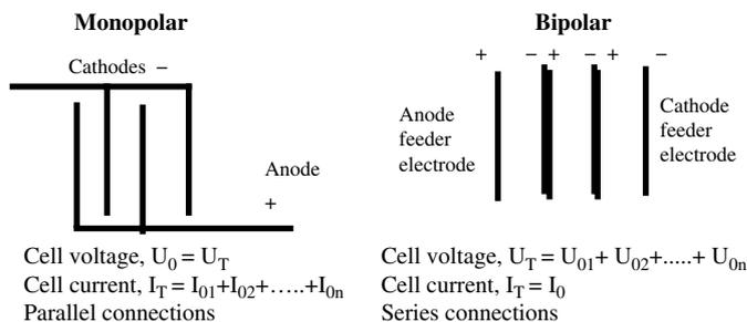
Fig. 2. Monopolar and bipolar electrode connections in the EC reactor (adapted from Jiang et al., 2002a).
