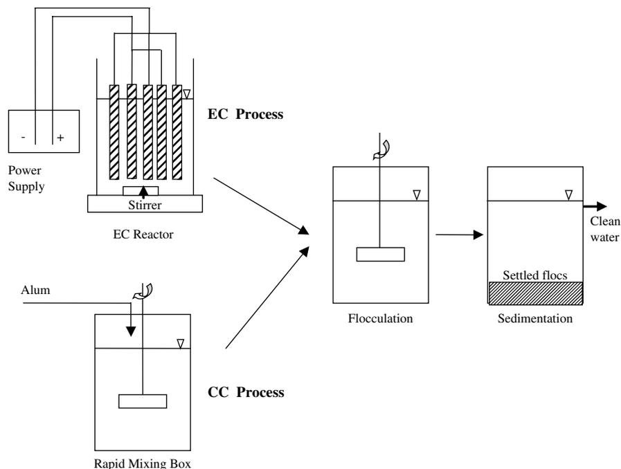
Fig. 7. Experimental set up for EC and CC processes (after Sivakumar et al., 2004).
