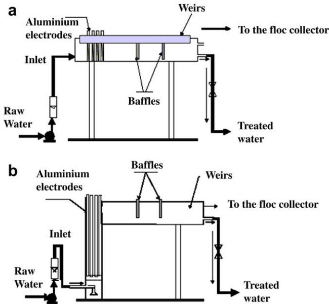
Fig. 6. Schematics of EC process [a] horizontal-flow electrocoagulation reactor and [b] up-flow electrocoagulation reactor (adapted from Jiang et al., 2002a).
