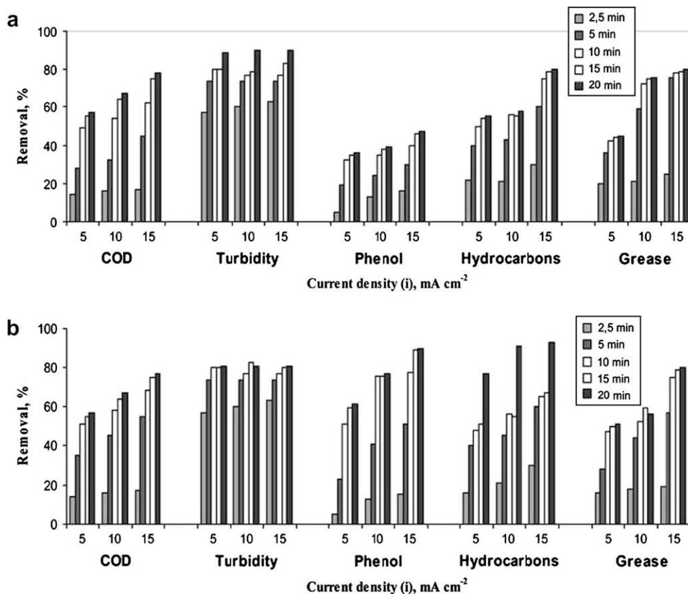
Fig. 5. Summary of EC performance for removal of the pollutants in different current densities and various electrolysis times [a] Fe electrode, [b] Al electrode (quoted in Dimiglo et al., 2004).
