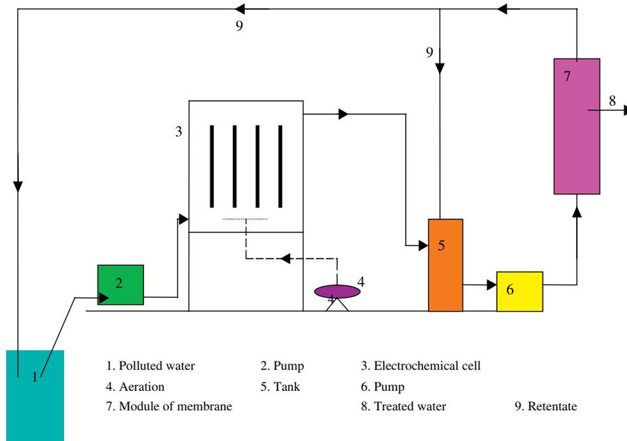
**Fig. 3.** Flow diagram of a hybrid process including electrocoagulation, flotation by aeration, and microfiltration processes for the municipal wastewater permeates removal (adapted from Pouet and Grasmick, 1995).
