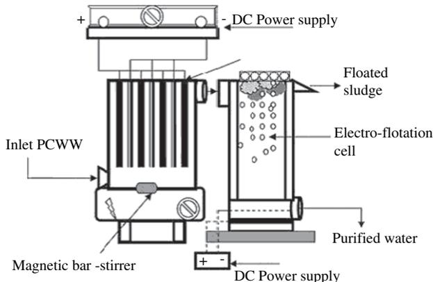
**Fig. 4.** Laboratory scale processes: (a) EF process, (b) EC and EF processes (adapted from Dimoglo et al., 2004).
