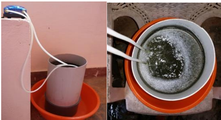
Fig 3: Aeration tank and airflow controlling devices
